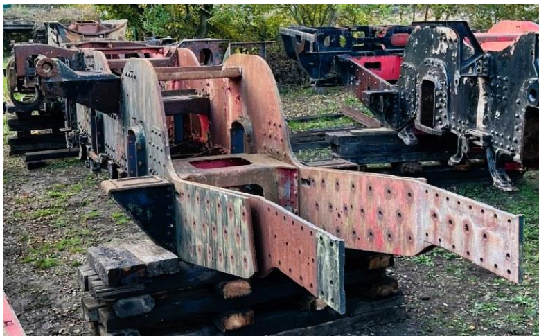
The frames of 34010 Sidmouth on arrival, rust had crept inside the steel sections.
